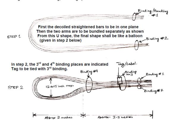
Ratio of balloon shape portion and straight portion is given above.
