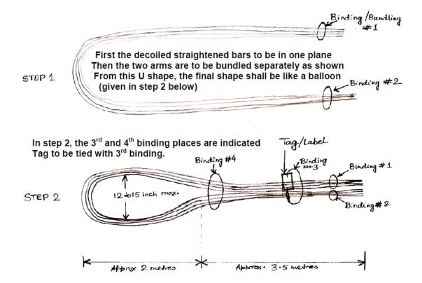
Diagram to show bending, bundling specifications for decoiled TMT Bars :
